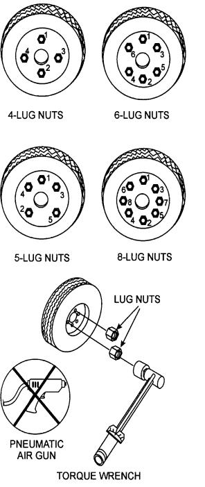
Figure 3. Wheel Lug Nuts Tightening Sequence
